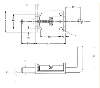
The Paneloc 779 Series spring latch features a 1/2" pin diameter and a closed knuckle for added durability and strength.
